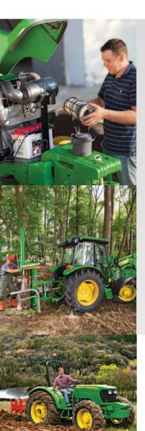
The 3-cylinder PowerTech M engine of the 5E Series tractor with its turbocharged and charge air cooled 2.9 litre capacity offers high performance as well as optimum fuel efficiency. Its integrated turbocharger compresses the intake air, thereby providing more oxygen for combustion. So you get more performance for less fuel. And because fuel consumption is reduced, the engine also meets Stage III A emission standards – and is kind on the environment.
