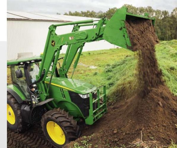
The twin-cartridge pressure relief valve on MSL / HSL loaders makes difficult tasks easier. One valve cartridge stops your loader stalling when you raise the boom with a dumped bucket; the other protects it from excessive forces during operations such as forward blading.
