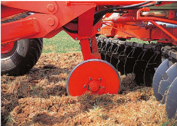
CRUMBLER ROLLER (only XS and XM2) Ø 550 - 75 kg/m
