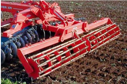
CRUMBLER ROLLER (only XS and XM2) Ø 550 - 75 kg/m
