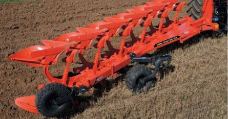
The wheel is equipped with a central pivot allowing it to automatically follow any changes in working width. The depth is adjusted by turnscrew (1) (or hydraulically with the possibility to adjust the depth differently on each side. The depth wheel can be mounted in many different positions along the beam in order to achieve the best
